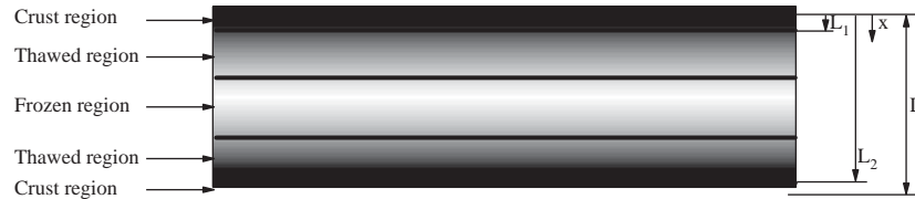
Fig. 1. A view of hamburger patty undergoing cooking (Adapted from Zorrilla & Singh, 2000).
