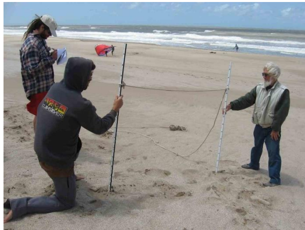
Figure 6. Measurement of beach profiles with the method developed by Bustos [30] .
