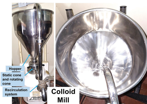
Figure 2: Colloid mill (CMX-65 model, CRYMA) used for nanofibrillation treatment
