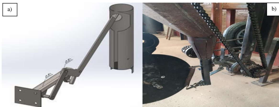
Figure 4: a) Detail of the planter mechanism. b) Planter mechanism of the prototype under development. Resistencia, Chaco, Argentina. 2017.
