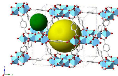
**Figure 8.** A schematic structure of MIL-125-NH<sub>2</sub>-(Ti) (color codes: gray bars: carbon backbone; red: oxygen; light-blue polyhedra: titanium centers) shows the two cage types (green and yellow spheres).
