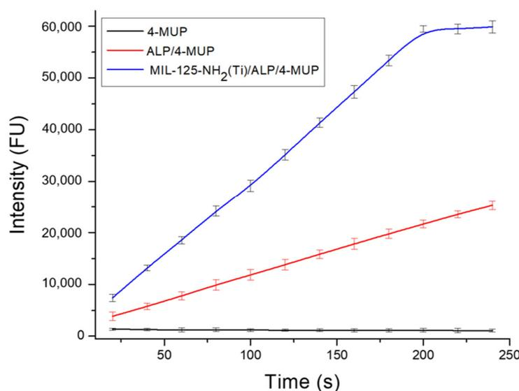
**Figure 13.** Fluorescence response at different incubation times of MIL-125-NH<sub>2</sub> (Ti)/ALP/4-MUP by modifying the paper support.
