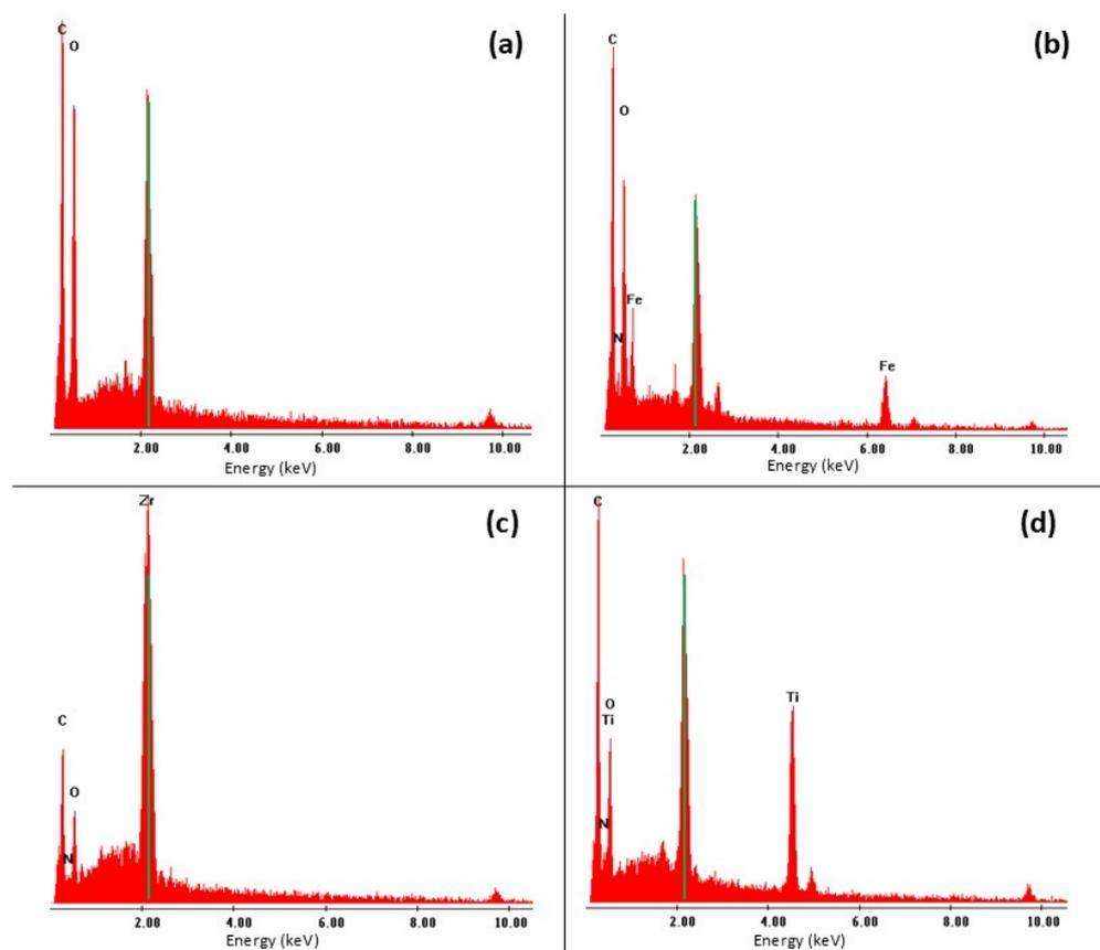
**Figure 4.** EDS spectra characterization: (a) unmodified paper surface, (b) paper surface modified with amino-functionalized MIL-101-NH<sub>2</sub> (Fe), (c) paper surface modified with amino-functionalized UiO-66-NH<sub>2</sub> (Zr), and (d) paper surface modified with amino-functionalized MIL-125-NH<sub>2</sub> (Ti). Note: the peak centered at 2.12 keV corresponds to the sputtered gold employed for the SEM technique.
