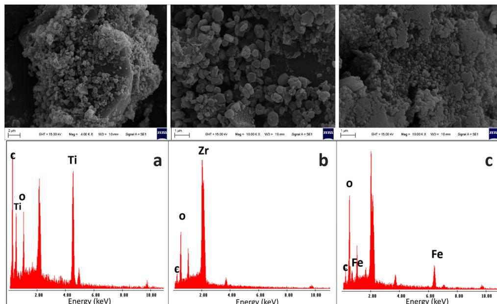
**Figure 2.** SEM image characterization: (a) MIL-125-NH<sub>2</sub> (Ti), (b) UiO-66-NH<sub>2</sub> (Zr), and (c) MIL-101-NH<sub>2</sub> (Fe).
