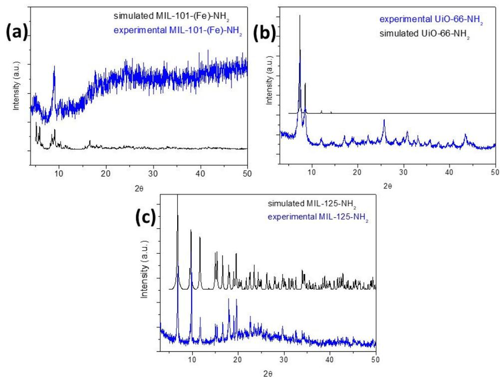
**Figure 5.** Experimental PXRD patterns of (a) MIL-101-NH<sub>2</sub> (Fe), (b) UiO-66-NH<sub>2</sub> (Zr), and (c) MIL-125-NH<sub>2</sub> (Ti) (blue lines) compared to the simulated diffractograms.
