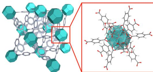
**Figure 7.** A schematic structure of UiO-66-NH<sub>2</sub> (Zr). The face-center-cubic UiO-66 structure type is composed of the metal node (aqua) and ligand (gray) with an atomic representation of the node and 12-connected 2-ATA linkers.
