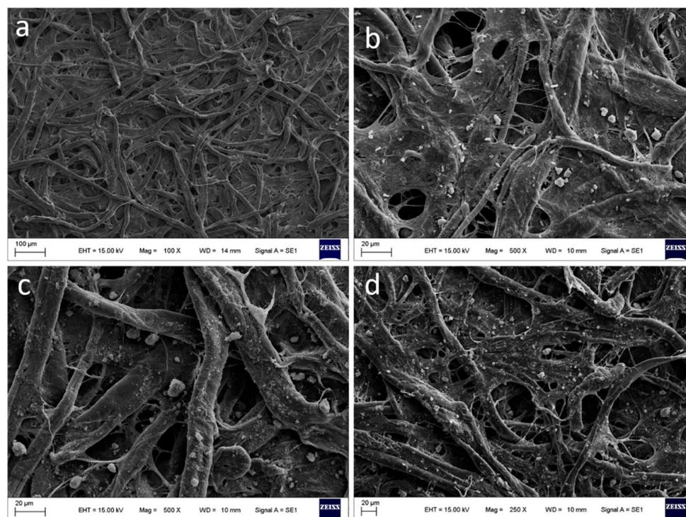
**Figure 3.** SEM image characterization: (a) unmodified paper surface, (b) paper surface modified with amino-functionalized MIL-101-NH<sub>2</sub> (Fe), (c) paper surface modified with amino-functionalized UiO-66-NH<sub>2</sub> (Zr), and (d) paper surface modified with amino-functionalized MIL-125-NH<sub>2</sub> (Ti).
