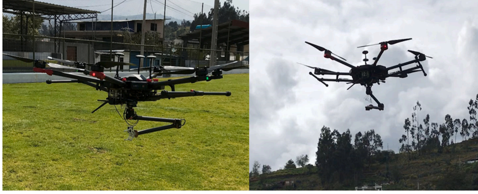
Fig. 7. Aerial manipulator robot used for the experimental tests.
