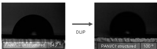
Figure 7. Contact angle of water drops deposited onto flat (left) and DLIP line structured (right) PANI films on PP.
