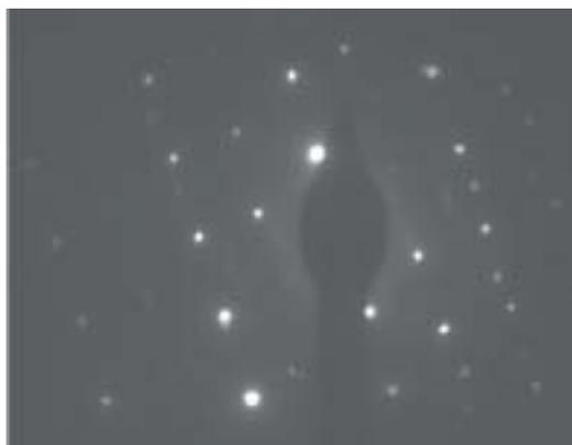
Figure 4: Electron diffraction pattern obtained from a large single crystal
