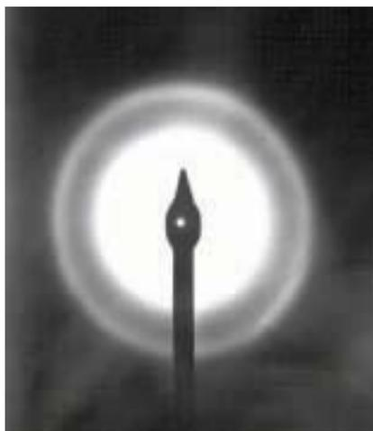
Figure 2: Electron diffraction pattern of an amorphous sample, see the circular rings
