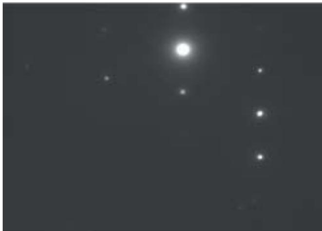
Figure 1: Electron diffraction pattern of a magnetized steel, see the central spot not coincident with the centre of the micrograph
