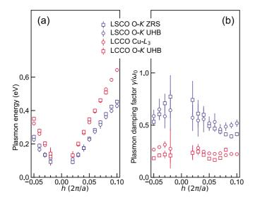
FIG. 3. Plasmon energies and lifetimes in LSCO and LCCO ( $\delta = 0.16$ ). (a) Plasmon energies extracted from fits to RIXS spectra at O *K*-edge ZRS and O *K*-edge UHB for LSCO and Cu  $L_3$ -edge and O *K*-edge UHB for LCCO. (b) Plasmon damping factor ( $\gamma / \omega_0$ ) extracted from the same fits.
