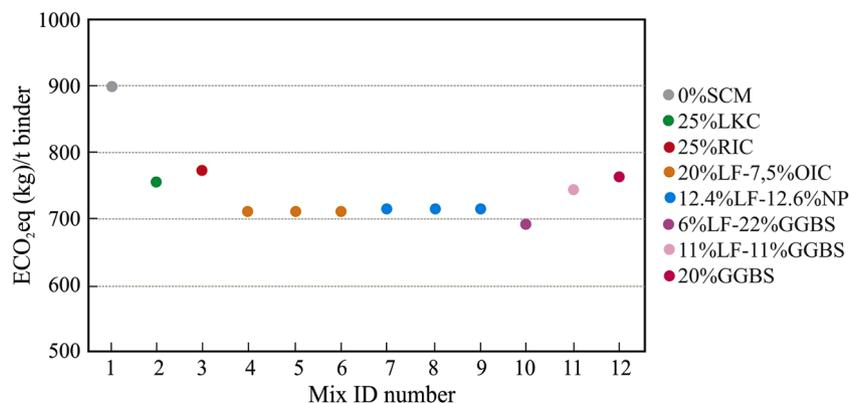
Fig. 1. ECO<sub>2</sub>eq (kg)/ton of binder.
