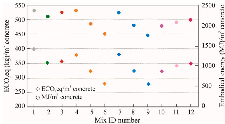
Fig. 2. ECO<sub>2</sub>eq (kg) and embodied energy (MJ) per m<sup>3</sup> of concrete.
