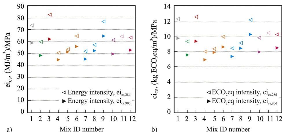
Fig. 5. a) Energy intensity and b) carbon intensity of concretes cured for 28 and 90 days.
