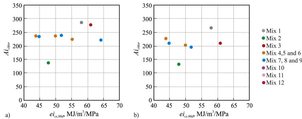
Fig. 6. Decision framework based on the  $A$ -index and energy intensity ( $ei_{cs,90}$ ) for chloride exposure of concretes cured for a) 28 days and b) 90 days.
