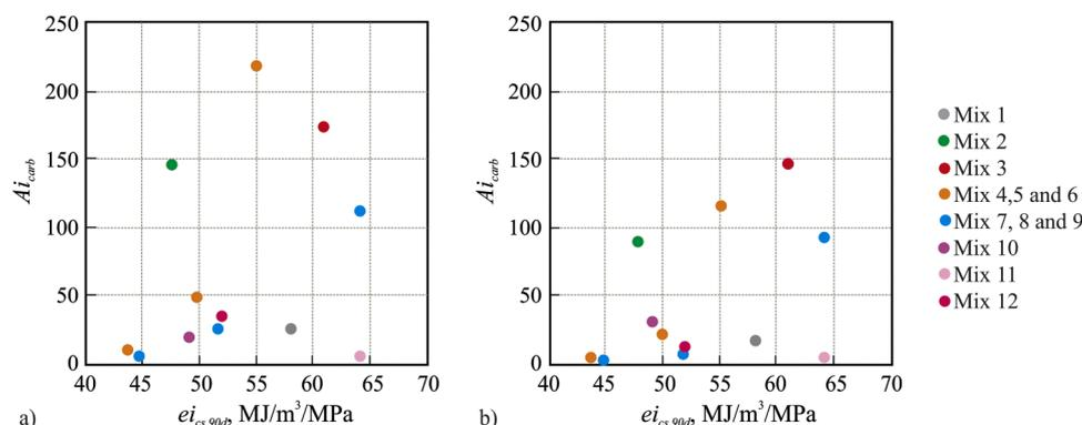
Fig. 7. Decision framework based on the  $A$ -index and energy intensity ( $ei_{cs,90}$ ) for carbonation of concretes cured for a) 7 days and b) 28 days.
