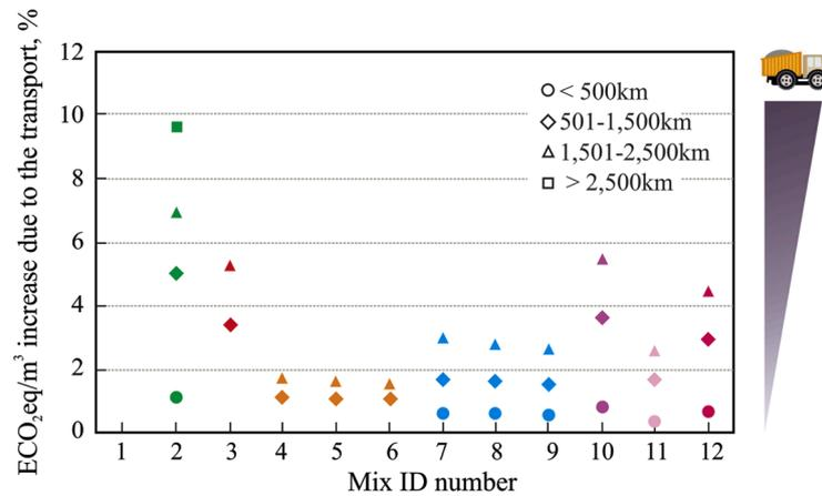
Fig. 4. Increase in  $\text{ECO}_2\text{eq}$  (kg) due to transport of the SCM.
