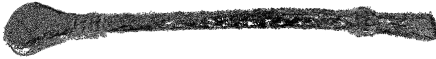
Fig. 2. 3D point cloud reconstruction of a metallic bombilla (straw) obtained with SFM photogrammetry and laser speckle.
