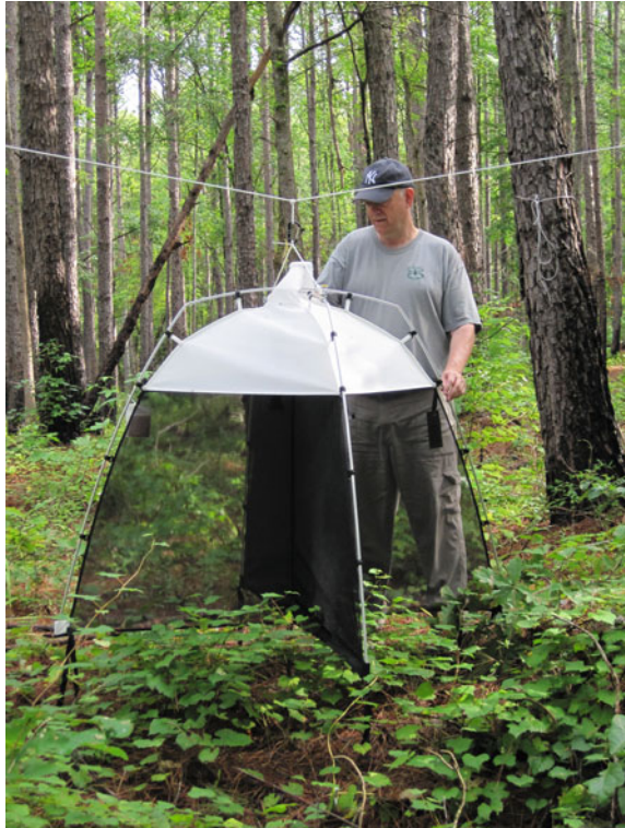
Fig. 19.5 A malaise trap for capturing flying insects. Credit: D. Miller, USDA Forest Service
