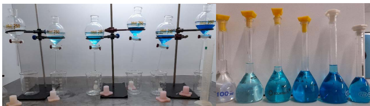
Figure 3: A) Chloroform extracts with washing solution. B) Calibration curve for measurement at 652 nm.
