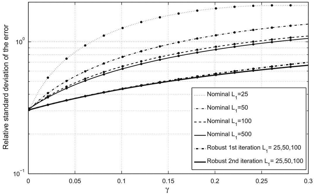
Fig. 10. Average value of the relative estimation error standard deviation for nominal and robust constrained design versus uncertainty amplitude.
