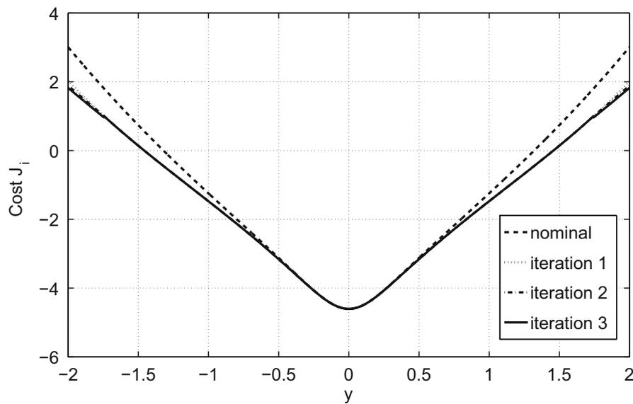
Fig. 4. Cost improvements for FIR  $y_k = u_k + v_k$  with  $\sigma_d^2 = 0.1$ ,  $\sigma_v^2 = 10^{-2}$ .
