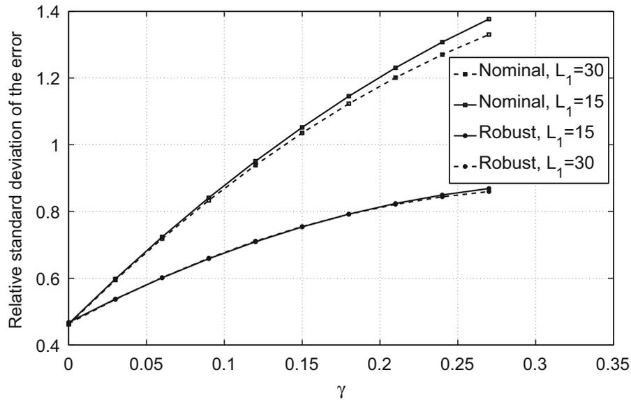
Fig. 8. Relative estimation error standard deviation for nominal and robust design versus amplitude of uncertainty.
