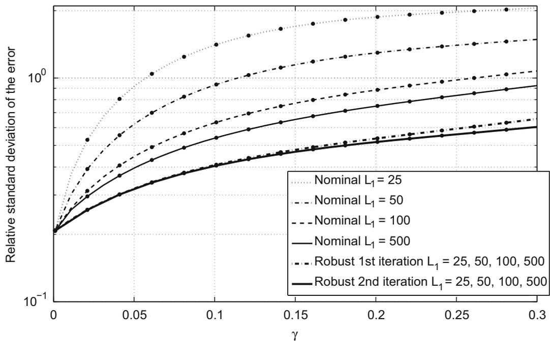
Fig. 9. Average value of the relative estimation error standard deviation for nominal and robust design versus uncertainty amplitude.
