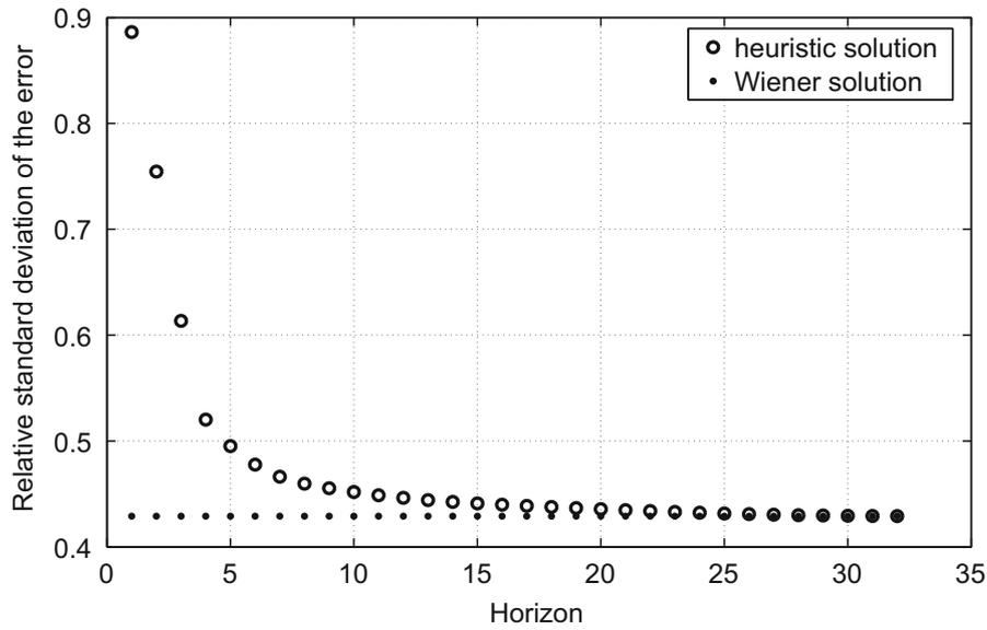
Fig. 6. Convergence of the heuristic cost to the Wiener solution as a function of the horizon length.
