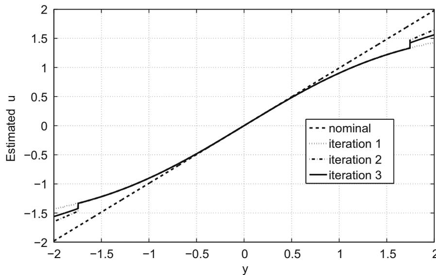
Fig. 5. Estimated values of  $u_k$  for FIR  $y_k = u_k + v_k$  with  $\sigma_d^2 = 0.1$ ,  $\sigma_v^2 = 10^{-2}$ .
