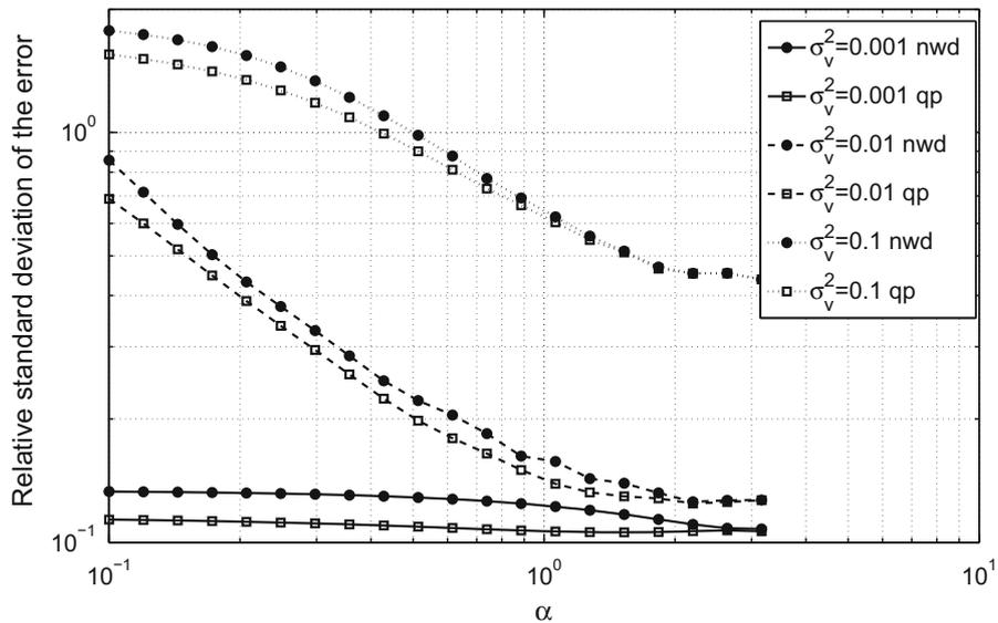
Fig. 7. Relative estimation error standard deviation for nominal with decision (nwd) and quadratic programme (qp) designs versus the half width  $\alpha$  of the truncated Gaussian.
