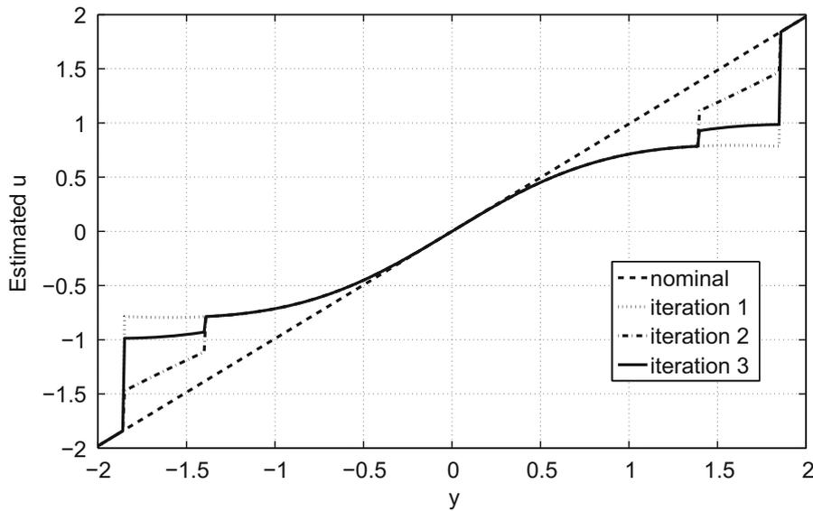
Fig. 3. Estimated values of  $u_k$  for FIR  $y_k = u_k + v_k$  with  $\sigma_d^2 = 0.4$ ,  $\sigma_v^2 = 10^{-2}$ .
