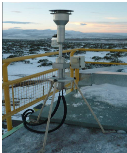
Fig. 1. Andersen-Graseby 240 dichotomous sampler at the sampling site: the roof of the FD building at Coihueco, Auger Observatory.
