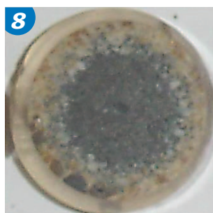
Fig. 8 Semidecarburized area of the B specimen (NC) tested at 1400 °C (air, 5 h)
