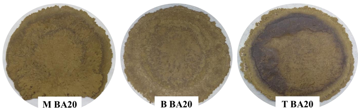
Figure 2. Sustainable materials obtained with bioadhesive formulations and yerba mate powder by thermo-compression. Monolayer (M), bilayer (B), and trilayer (T) systems using BA20 adhesive. Nomenclature BA = 1,2,3,4 butane-tetracarboxylic acid, the next
