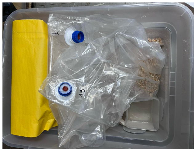
Figure 1. Plastic box with two plastic bags (transparent, for modified and self-modified atmosphere treatments) and one poly-paper bag (yellow, for normal atmosphere treatment), and a container with glycerol solution. The valve with the rubber septum can be seen in the corner of each bag.
