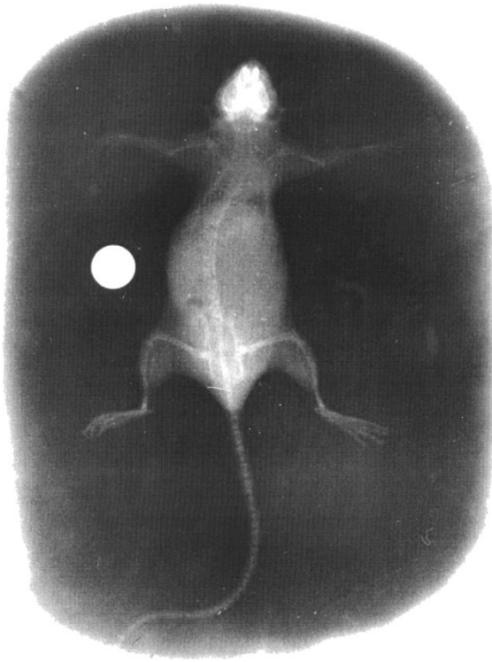
Fig. 4. Radiograph of a live mouse, taken with an X-ray flash 10-ns exposure time. It is obtained in a single shot of PACO device. White circle corresponds to an iron bar of 1 cm diameter and 1 cm length.
