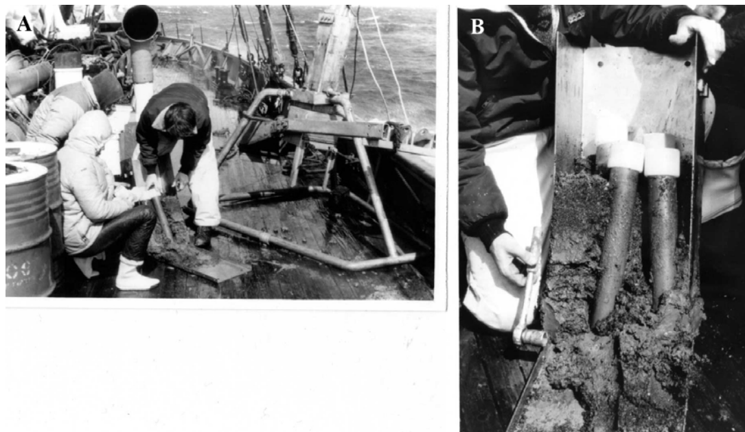
Figure 4. A) Box core device on deck of the El Austral vessel. B) Subsampling the box core with plastic tubes.
