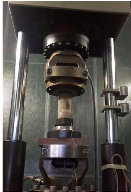
Figure 2. Zwick Amsler 400 HFP 5100 Vibrophore equipment. Schematic diagram of equipment and test specimen.
