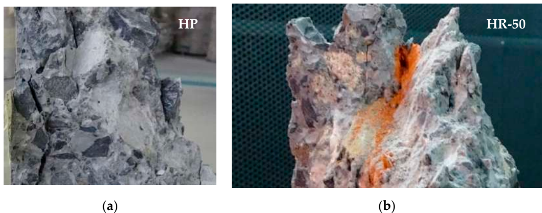
Figure 13. Fracture surface detail of samples broken during fatigue tests: HP sample (a) and HR-50 sample (b).
