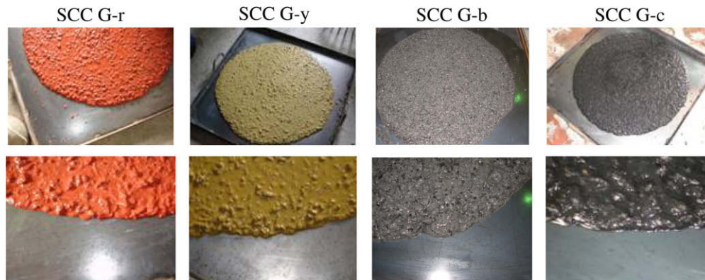
Fig. 7. Slump-flow tests of C-SCC with cement G.
