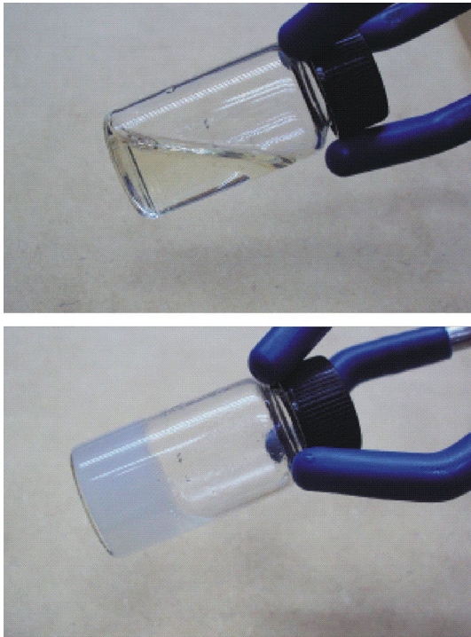
Fig. 2 Chitosan/ \beta -glycerophosphate formulation at room temperature ( top ) and after solution-to-gel transition at 37 °C ( bottom )
