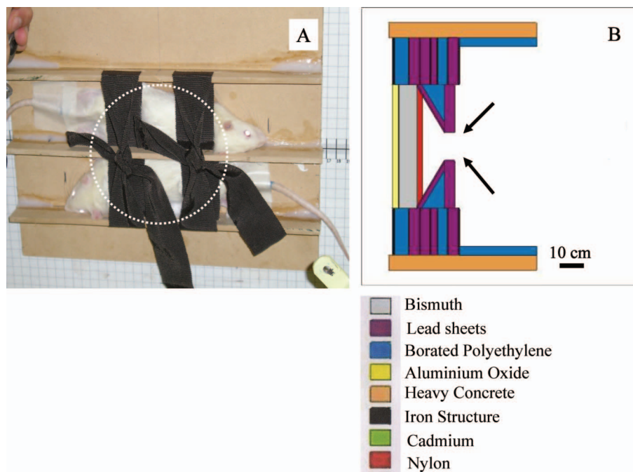
Figure 1. Rats positioned at the RA-6 beam port for local irradiation. The abdomen is placed at the center of the beam port (15 cm in diameter, indicated by the white circle) (A). The head and posterior end of the body of the rat remain radially outside of the beam, shielded by the lead and borated polyethylene beam aperture delimiter schematically shown in (B). The arrows in B indicate the position of the beam port.
