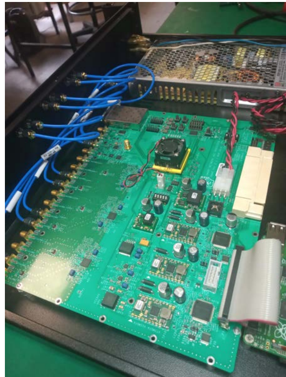
Fig. 7. SNAP board for Pathfinder digitizer.
