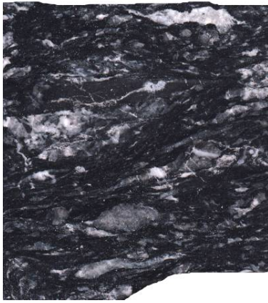
Figure 3. Hand sample showing a gneiss texture with melanocratic bands, composed by white micas, and leucocratic sectors dominated by quartz and feldspars, and affected by metamorphism.
