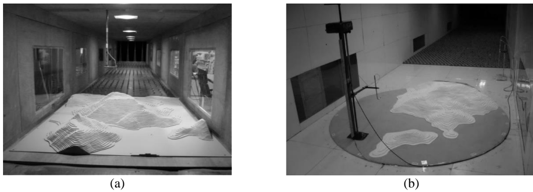
Fig. 16 Complex topography models inside the wind tunnels in Brazil (a) and Argentina (b)
