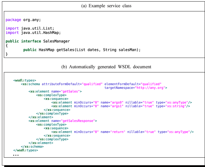
Figure 9 Automatic WSDL generation with ‘Whatever types’ anti-pattern occurrences (see online version for colours)
