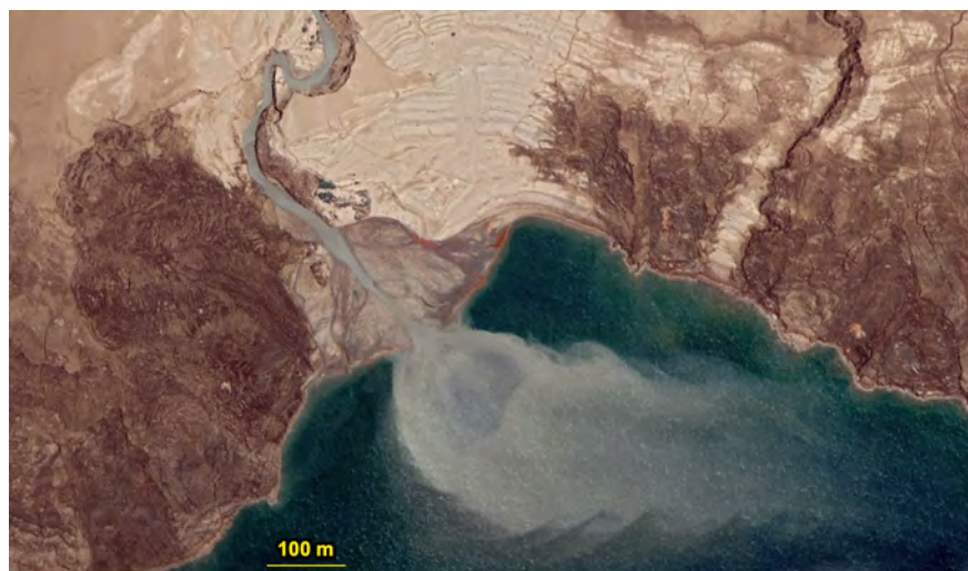
FIGURE 7 Buoyant plume of the Jordan River over the Dead Sea: Note that, because of the excess of buoyancy induced by the high \Delta\rho_b , part of the river momentum is transferred to the overflow, resulting in a narrow and elongated buoyant plume. Image from Google Earth, June 2019.
