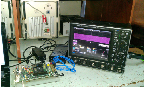
Fig. 6. Laboratory set up. FPGA and Lecroy logic analyzer.
