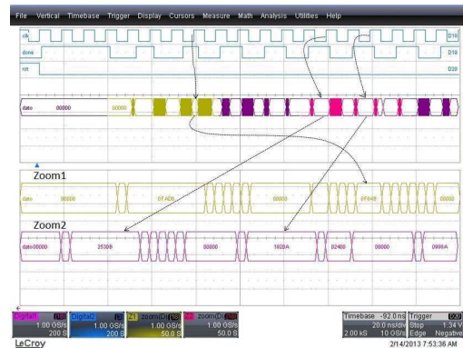
Fig. 5. PWL output capture. The bottom part shows an output zoom. We can see the output throughput is half the clock frequency.
