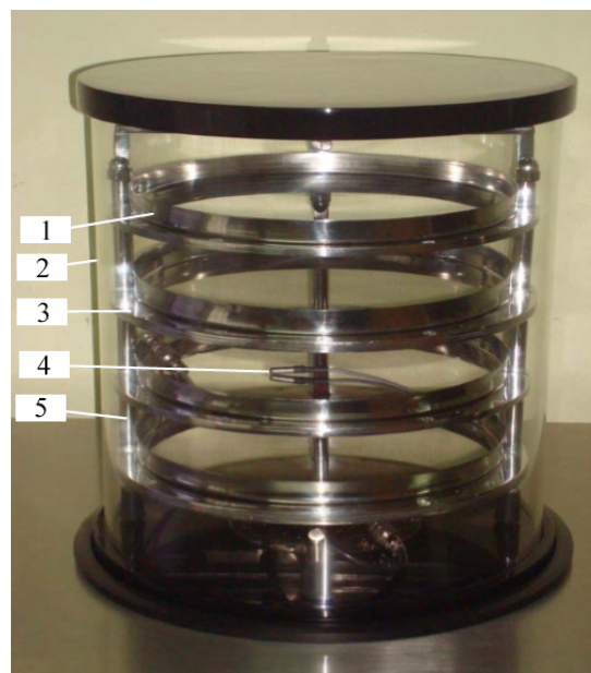
Figure 2: Vacuum chamber of the Rifcor L-A-B4-C Freeze dryer. 1. Tray; 2. Transparent vacuum chamber; 3. Temperature-controlled shelf; 4. Product temperature sensor; 5. Framework supporting the structure of the shelves under high vacuum.
