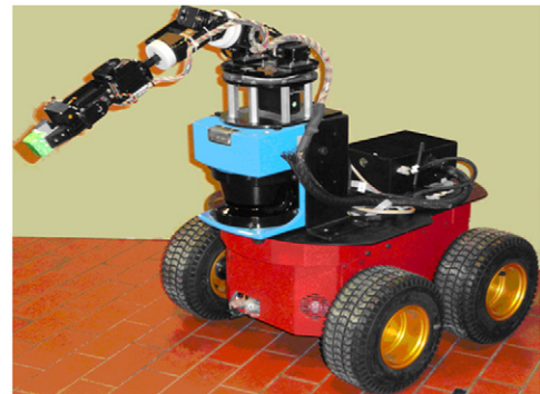
Fig. 8. Mobile manipulator used in the experiments. Mobile platform Pioneer 3-AT, and robotic arm Cyton Alpha 7 dof.
