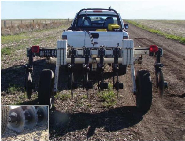
Fig. 2. Veris 3100 coulter-based apparent soil electrical conductivity sensor.
