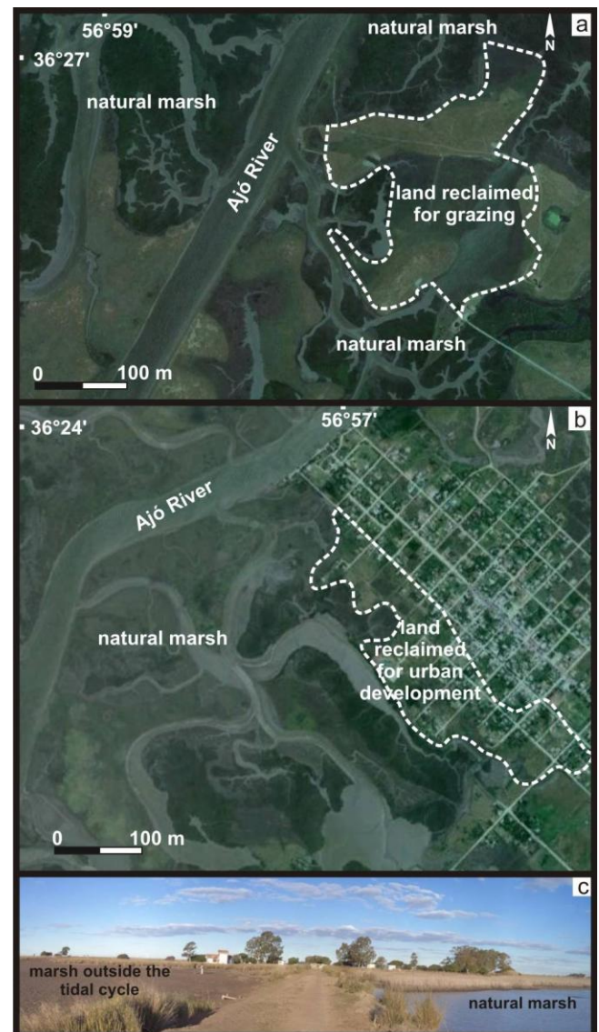
Figure 3. (a) Image of the marsh area with levees to reclaim low-lying ground for grazing; (b) image of the marsh with levees in the urban area to extend constructions; (c) photo of the levee appearing in image (a), in whose centre a levee excluding a section of the marsh from the tidal cycle (to the left of the image) can be observed.
