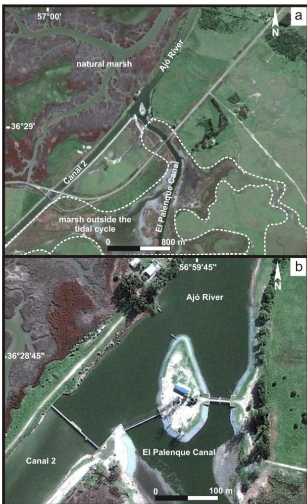
Figure 5. (a) Image of the marsh area excluded from the tidal cycle due to the presence of floodgates in the canals; (b) detail of the floodgates
