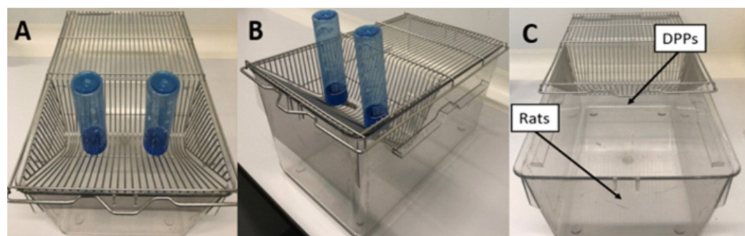
Figure 3. Cage and bottle arrangement in the two-bottle-choice test. A. Upper frontal vision. B. Lateral frontal vision. C. Positioning of Dustless precision pellets (DPPs) and rats during the binge eating (BE) episode.
