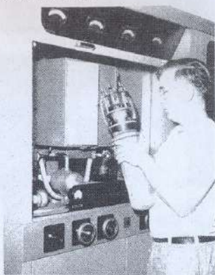
Fig. 22. Installing the finished tube
