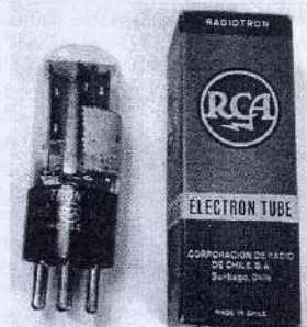
Figs. 3A and 3B. Chilean tubes with familiar RCA graphics. The lower one is a late-vintage 80 in a T9 bulb.
