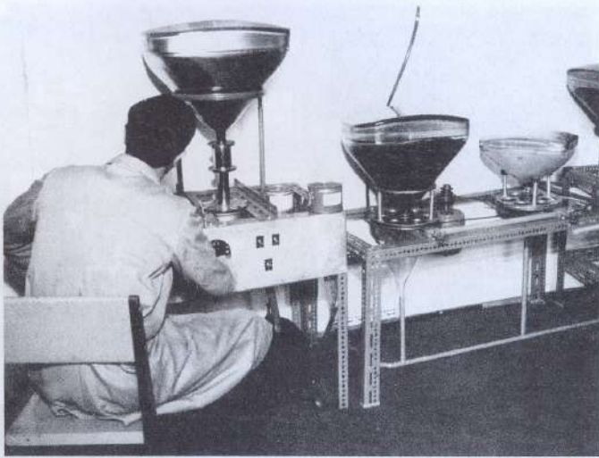
Aluminizing and lacquering the bulb
