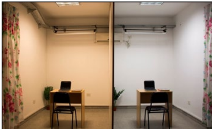
Figure 3. The lab setup: the warm (3000 K) and cool (4000) CCT at the higher level (front wall light ON).
