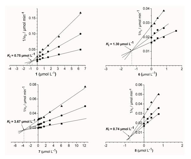
**Figure 5.** Dixon plots for determination of the type of inhibition and inhibition constants ( $K_i$ ) for compounds **1**, **6**, **7**, and **8** towards glutathione *S*-transferase from horse liver (GST). The concentrations of the substrate 1-chloro-2,4-dinitrobenzene were 200  $\mu$ M ( $\blacktriangle$ ), 400  $\mu$ M ( $\bullet$ ), and 800  $\mu$ M ( $\blacksquare$ ).
