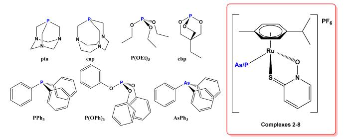
**Figure 2.** Phosphine, phosphite, and triphenyarsine ligands used in this study and the general structure of synthesized complexes **2–8**.
