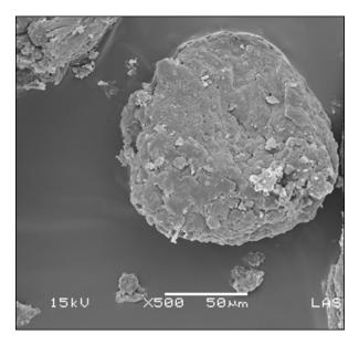
**Figure 1.** Scanning electron micrograph (SEM) of an alginate microcapsule with *B. bassiana* conidia, scale 50 μm.
