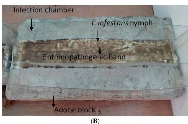
**Figure 2.** (**A**) Bioassay prototype for triatomine exposure to bioinsecticidal formulations. (**B**) Triatomines were exposed for 1 min on the entomopathogenic band for follow-up post-exposure.
