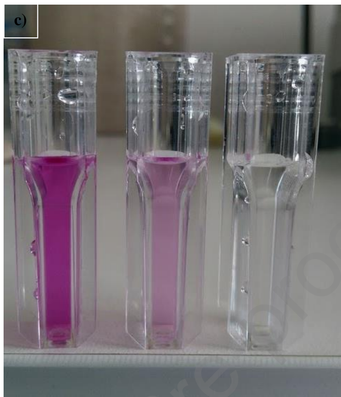
Figure 10. \text{Cr}^{6+} concentration profile for each material in the photoelectrochemical circuit under different conditions. a) irradiation without the presence of EDTA. b) irradiation with the presence of 4 \text{ mg L}^{-1} EDTA. c) photograph showing the decrease in concentration of \text{Cr}^{6+} through the photocatalytic process. For all cases the initial \text{Cr}^{6+} was 1 \text{ mg L}^{-1} at pH 2.0.
