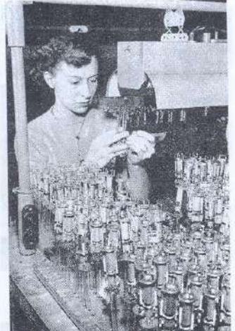
An inspector examines the assembly of an electron gun, to assure that this fundamental element of a picture tube meets rigid specifications.
