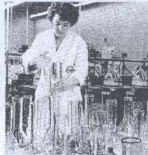
An operator pours phosphor solution into 7-inch picture tubes.
