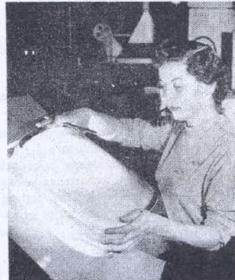
Exposure to a powerful light allows this inspector to give the screen surface of the picture tube a final inspection before shipment.
