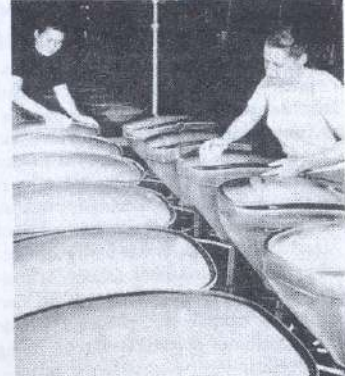
Faceplates of metal-shell and glass rectangular kinescopes are carefully cleaned before the tubes move on to the next step in production.
