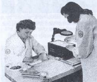
Worker examines a mesh screen, to be used in an orthicon, for blemishes.
