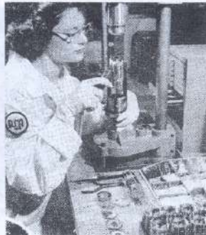
Cathode-ray "gun" is added to an image-orthicon camera tube.
