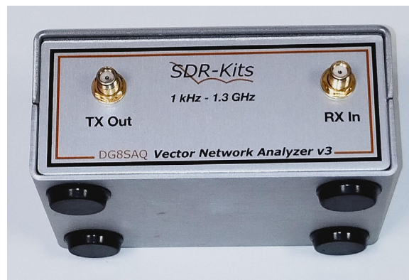
Fig. 6. VNWA for measurement of S parameters.
