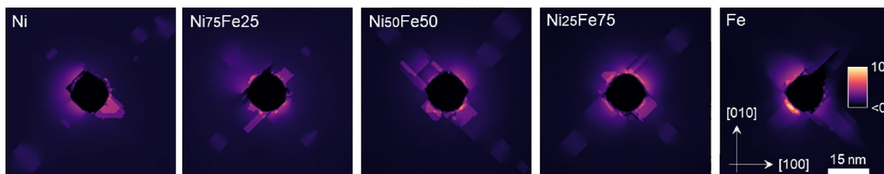
Figure 13. Top view of the residual surface imprints for the samples investigated. Color scale indicates height above the original surface, in Å units.
