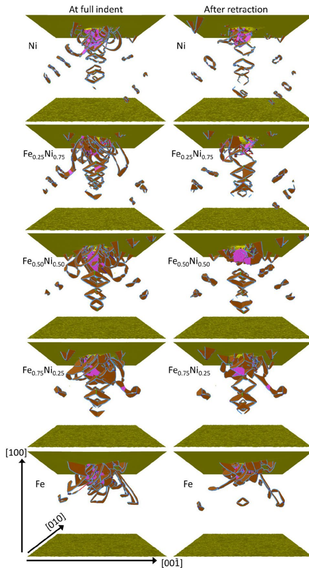
Figure 7. Snapshots showing the stacking-fault planes (brown) and twin boundaries (pink) in elemental Fe and Ni and several random \text{Fe}_x\text{Ni}_{1-x} alloys at full indentation (left) and after retraction of the indenter (right). The crystallographic orientations of the sample are indicated in the bottommost panel. Slip occurs on \{111\} planes in \langle 110 \rangle direction. Twin boundaries are \{111\} planes and the twin direction is \langle 112 \rangle .
