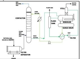
Figure 2.Diagram of a Typical Process Natural Gas Dehydration with TEG.
