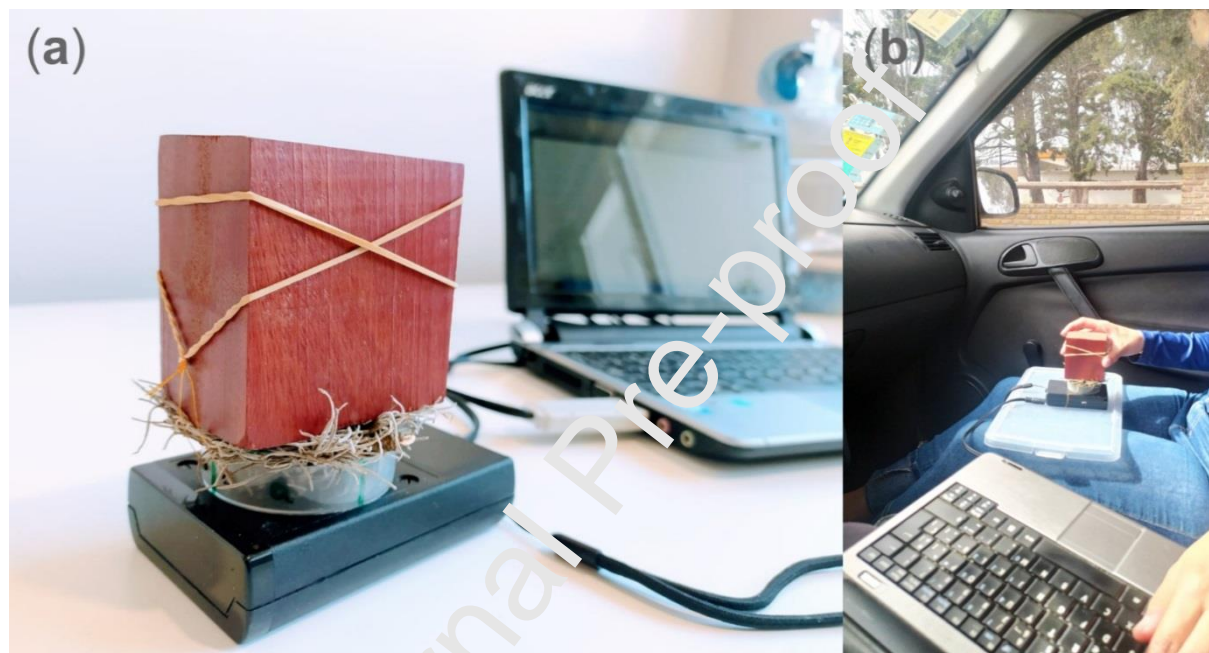
Fig. 2. In situ magnetic susceptibility measurements ( \kappa_{is} ) using the protocol proposed by Chaparro (2021) and Butraño Posada & Chaparro (2022). Ten readings were performed by contact between a high-resolution range portable meter SM 30 (ZH Instruments Ltd.) and a Petri plastic dish where the plant is pressed with a block of wood to increase the plant's surface contact (PWM). \kappa_{is} readings at the laboratory (a) and inside a car (b) close to the sampling site.
