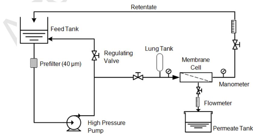
Fig. 1: Schematic diagram of the experimental set-up for nanofiltration.
