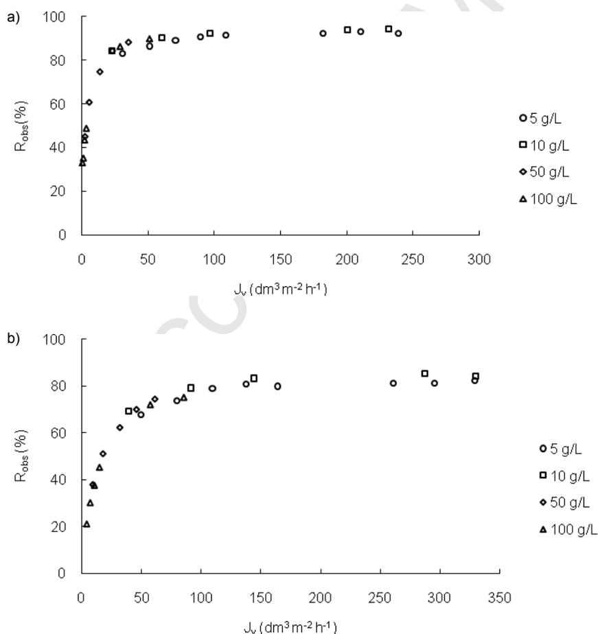
Fig.4: Observed rejections ( $R_{obs}$ ) of glucose solutions (5, 10, 50, and 100 g/L) as function of the permeate flux ( $J_v$ ) for a) DK and b) DL membranes.
