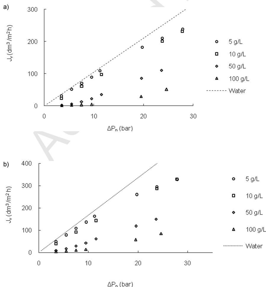
Fig. 3: Permeate flux ( $J_v$ ) for pure water and glucose solutions (5, 10, 50, and 100 g/L) using a) DK and b) DL membranes.
