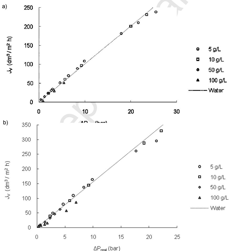
Fig. 6: Permeate flux ( $J_v$ ) of water and glucose solutions (5, 10, 50, and 100 g/L) as a function of the real driving force ( $\Delta P_{real}$ ) for a) DK and b) DL membranes.
