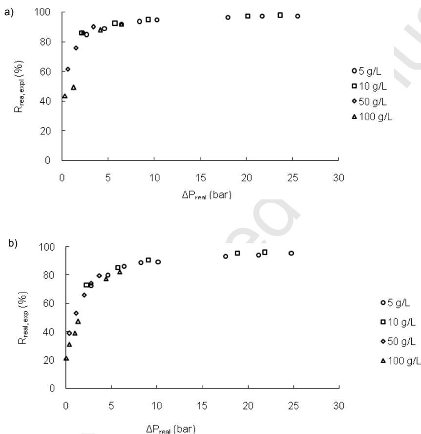
Fig. 7: Experimental real rejection ( $R_{real,exp}$ ) of glucose for different concentrations (5, 10, 50, and 100 g/L) as a function of the real driving force ( $\Delta P_{real}$ ) for a) DK and b) DL membranes.
