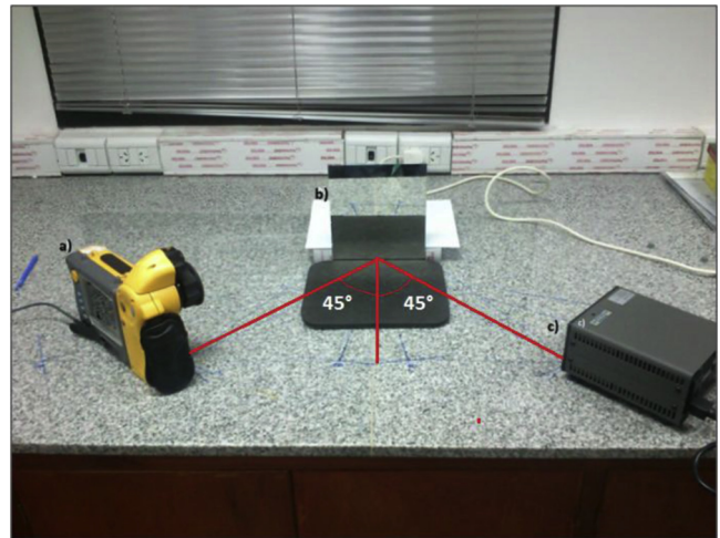
Fig. 5. Experimental layout. (a) Thermographic camera, (b) specular target, and (c) infrared radiation source, positioned to make measurements for \theta = 45^\circ .
