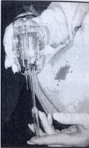
Bulb sealed to stem
